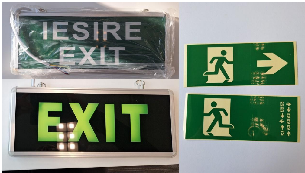
Figure 2 Examples of emergency exit signs the products were sold with. These signs are non-compliant with the relevant standard (EN 1838 Lighting applications - Emergency lighting for buildings)
