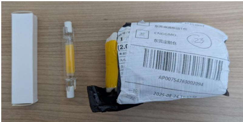
Figure 3 Samples of R7s lamps received. The packaging was often missing and, when present, was blank with no markings, no relevant safety information nor manufacturer's information.
